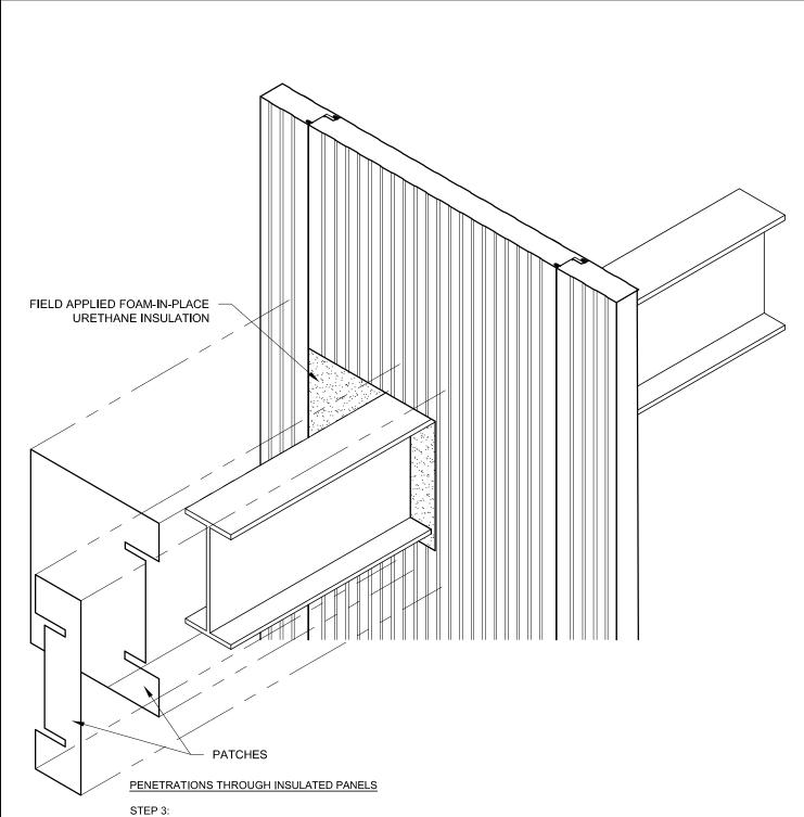
FILL NOTCH WITH FOAM-IN-PLACE URETHANE INSULATION, FIELD CUT ANY FOAM THAT EXPANDS BEYOND THE FACE OF THE INSULATED PANEL SKIN
